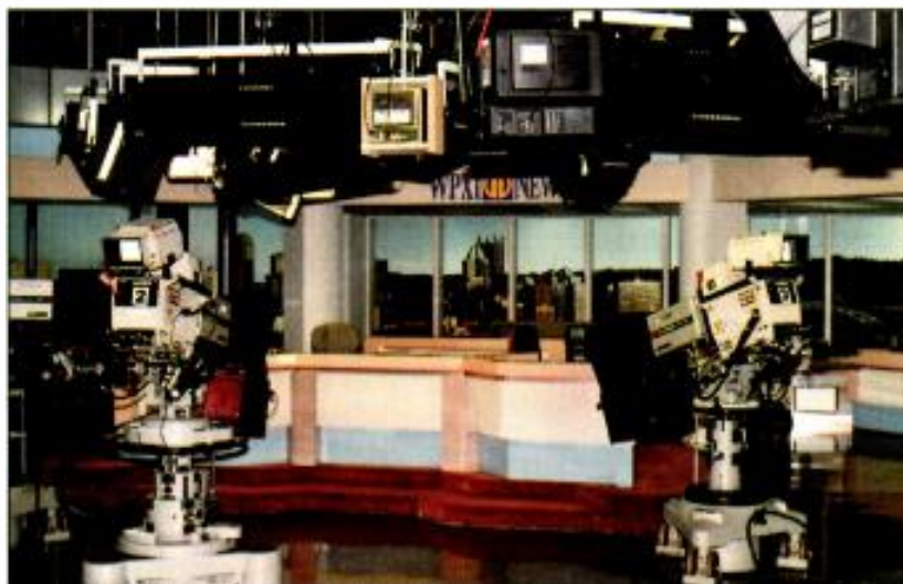
Among the items that need to be considered when planning for HDTV are studio sets and lighting. Grid height and set size may have to be increased to accommodate the change in aspect ratio. (Photos courtesy of KSBH Architects and WPXI, Pittsburgh.)
