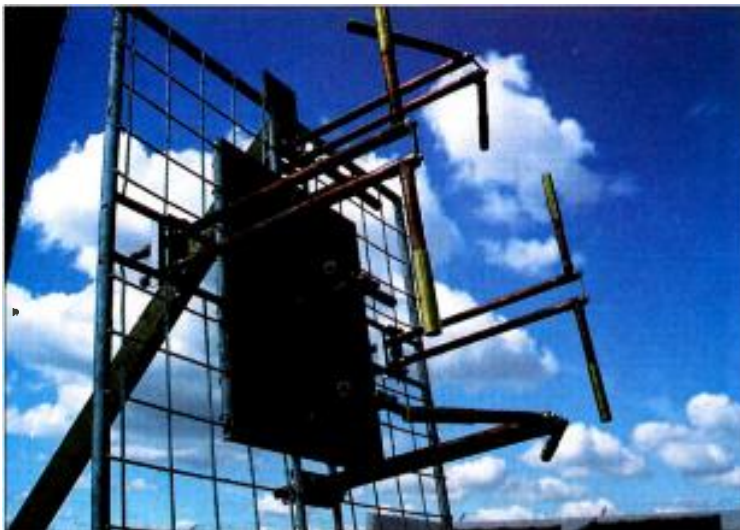
Among the possible HDTV antenna types is this dual-mode panel from Jampro. These units can be used in any application where aperture and/or windload are critical factors.
