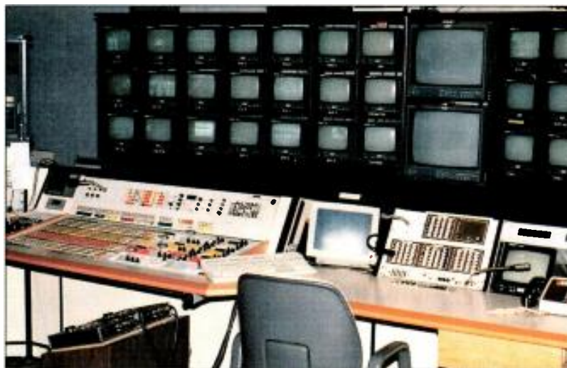
HDTV's 16:9 aspect ratio will affect studio control rooms. In addition to installing new equipment, the size and shape of monitor walls will have to be addressed.
